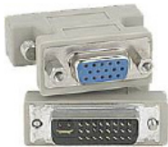
DVI interface on 700A outputs analog signals only, using included DVI-to-VGA adaptor.
