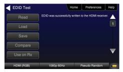
EDID Sink Testing – Run an EDID functional test on an HDMI HDTV and/or an A/V receiver to verify EDID checksum, header, and HDMI video and audio support. View entire EDID contents. Run portions of the EDID compliance test
