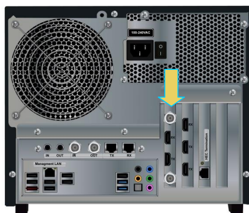
Previous 980 HDMI Protocol Analyzer board rev.
