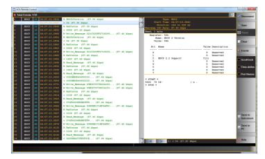
Auxiliary Channel Analyzer showing HDCP 2.2 transactions
