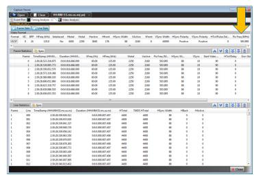
Timing Analyzer showing parameters for 600MHz format
