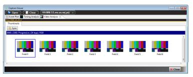
HDMI 2.0 source capture of video frames (SMPTEBar Pattern)
