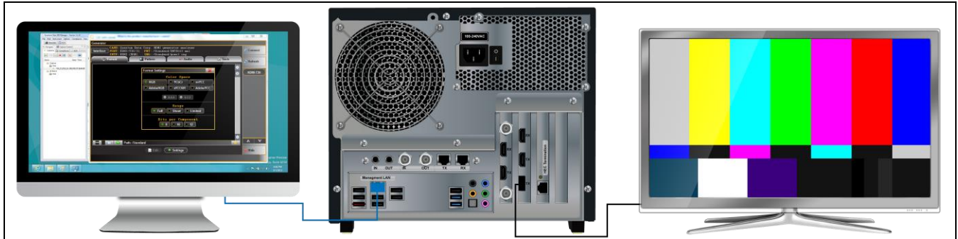
Connection for video testing Tx2 – 980 example
