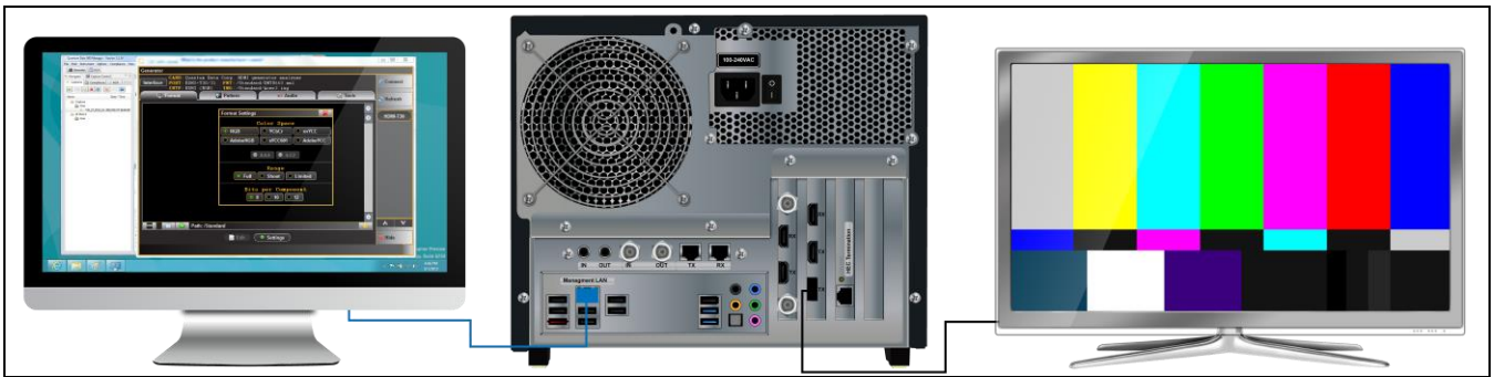
Connection for video testing (e.g. Tx2) – 980 example
